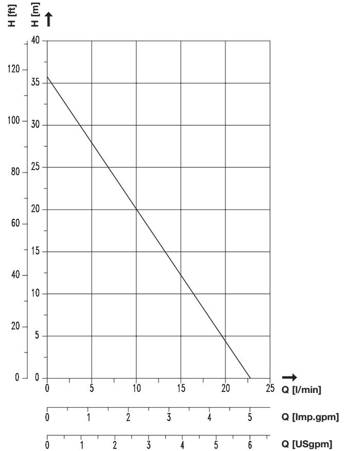
The data apply to fluids with a viscosity of 1 mm<sup>2</sup>/s at a density of 1 kg/dm<sup>3</sup>
